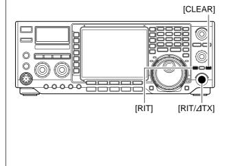
When RIT and  $\Delta$ TX are ON at the same time, the [RIT/ $\Delta$ TX] control shifts both the transmit and receive frequencies from the displayed frequency at the same time.
