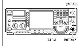
When RIT and  $\Delta$ TX are ON at the same time, the [RIT/ $\Delta$ TX] control shifts both the transmit and receive frequencies from the displayed frequency at the same time.
