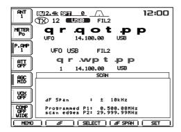
④ Select the desired memory channel to set as a select memory channel. ⑤ Push [(F-3)SELECT] to set the memory channel as a select memory or not.
