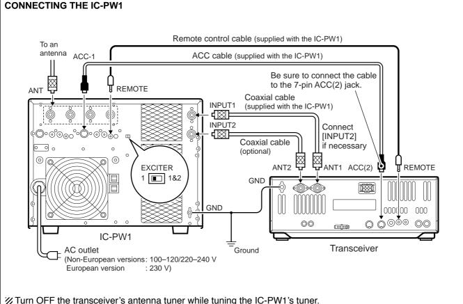
I'V Turn OFF the transceiver's antenna tuner while tuning the IC-PW1's tuner.
