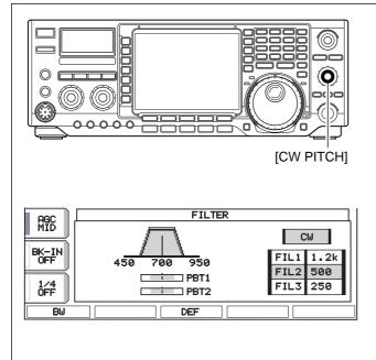
The received CW audio pitch and monitored CW audio can be adjusted to suit your preference (300 to 900 Hz in 25 Hz steps) without changing the operating frequency.
