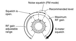
•When functioning as RF gain control (Squelch is fixed open; SSB, CW, RTTY only)
