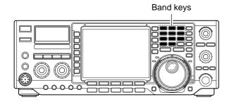
The triple band stacking register provides 3 memories in one band. 3 sets of a frequency and operating mode on each band are automatically stored when used.
