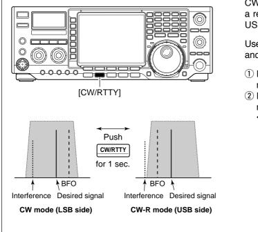
CW-R (CW Reverse) mode receives CW signals with a reverse side CW carrier point like that of LSB and USB modes.
