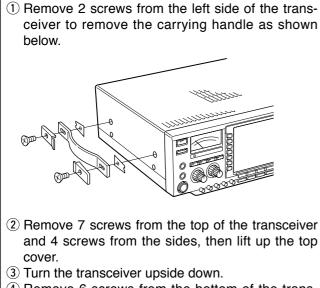
④ Remove 6 screws from the bottom of the transceiver, then lift up the bottom cover.
