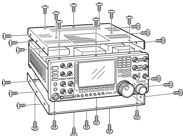
Follow the case opening procedures shown here when you want to replace the clock backup battery or internal fuse.
