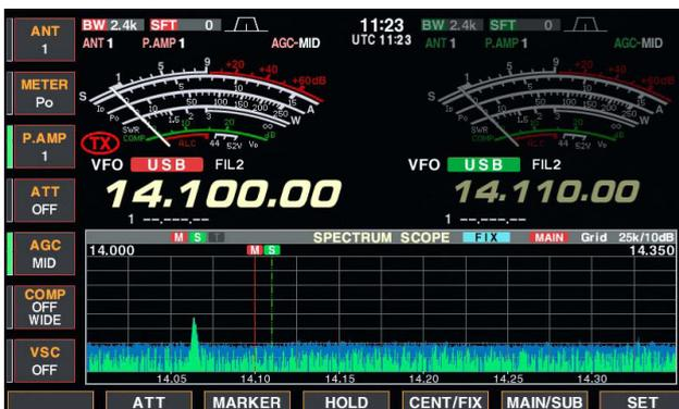
Displays signals within the specified frequency range. The selected frequency band conditions can be observed at a glance when using this mode.
