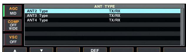
When no antenna is connected to [ANT2], [ANT3], and/or [ANT4], these antenna connectors can be deactivated— deleting the antenna number from selection. This prevent the transceiver from accidentally transmitting into an empty antenna connector. In addition, a receive-only antenna can be specified for [ANT4].
