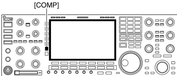
➔ During USB or LSB mode selection, push [COMP] for 1 sec. several times to select the desired transmit filter width from wide, middle and narrow.
