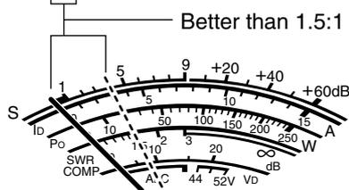
The SWR meter indicates the SWR over the transmission line in all modes.
