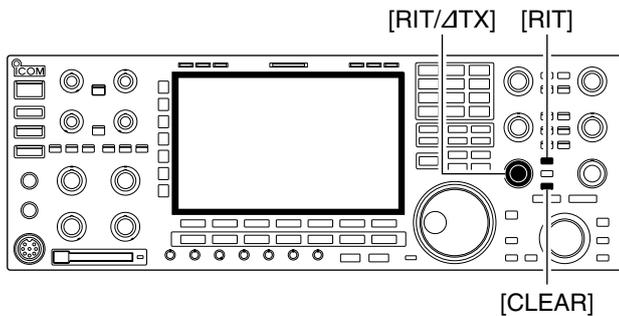
The RIT (Receive Increment Tuning) function compensates for off-frequencies of the communicating station.
