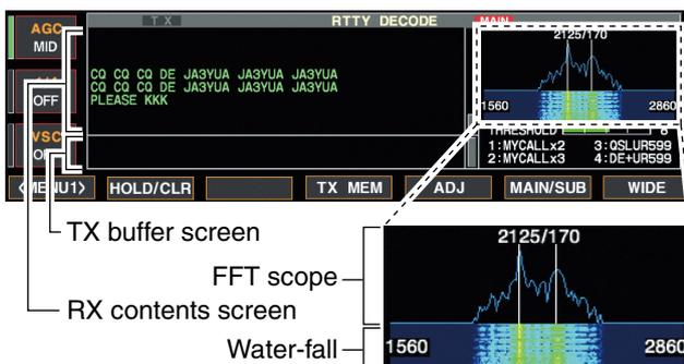
A DSP-based high-quality Baudot RTTY encoder/decoder is built-in to the IC-7800. When connecting a PC keyboard (p. 2-6), RTTY operation can be performed without an external RTTY terminal, TNC or PC.
