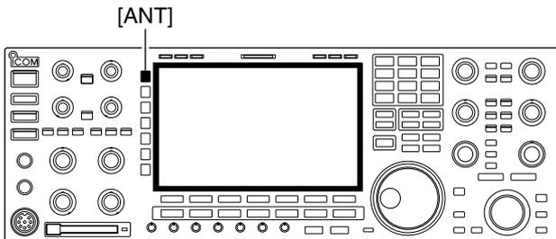
When “Manual” is selected, you can use the all antenna connectors, [ANT1] [ANT2], [ANT3] and [ANT4], however, band memory does not function. In this case you must select an antenna manually.
