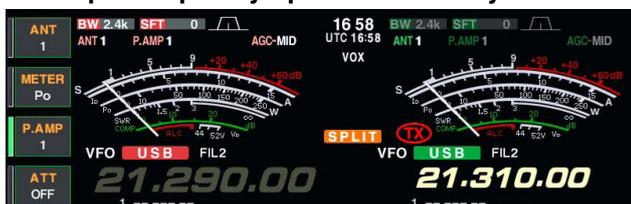
Split frequency operation allows you to transmit and receive in the same mode on two different frequencies. The split frequency operation is performed using 2 frequencies on the main and sub readouts.
