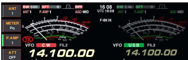
During full break-in operation, the transceiver automatically selects transmit while keying and returns to receive immediately after keying is finished.
