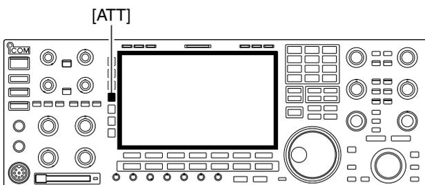
The attenuator prevents a desired signal from distortion when very strong signals are near the desired frequency or when very strong electric fields, such as from broadcasting stations, are near your location.
