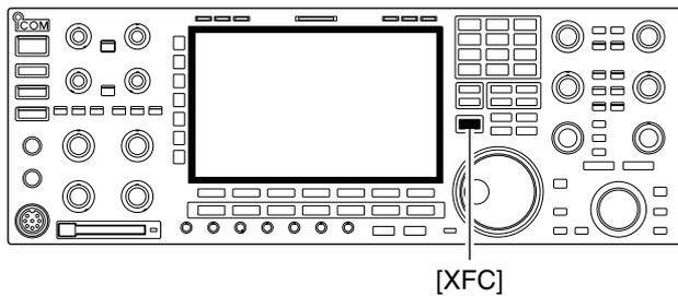
When the RIT function is ON, pushing and holding [XFC] allows you to monitor the operating frequency directly (RIT is temporarily cancelled).
