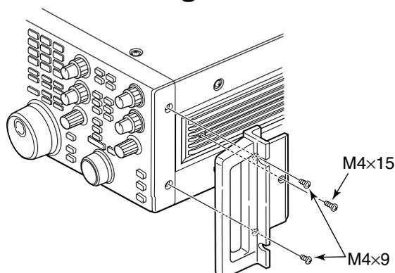
Remove the four screws from both sides of the front panel and the two screws from both sides of the side panel, then attach the rack mounting handles to the sides of the transceiver using the supplied screws.
