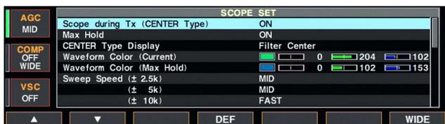
This set mode is used to set the waveform color, sweeping speed, scope range for fix mode, etc.
