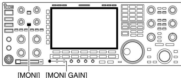
The monitor function allows you to monitor your transmit IF signals in any mode. Use this to check voice characteristics while adjusting SSB transmit parameter. (p. 12-4) The CW sidetone functions regardless of the [MONI] switch setting.
