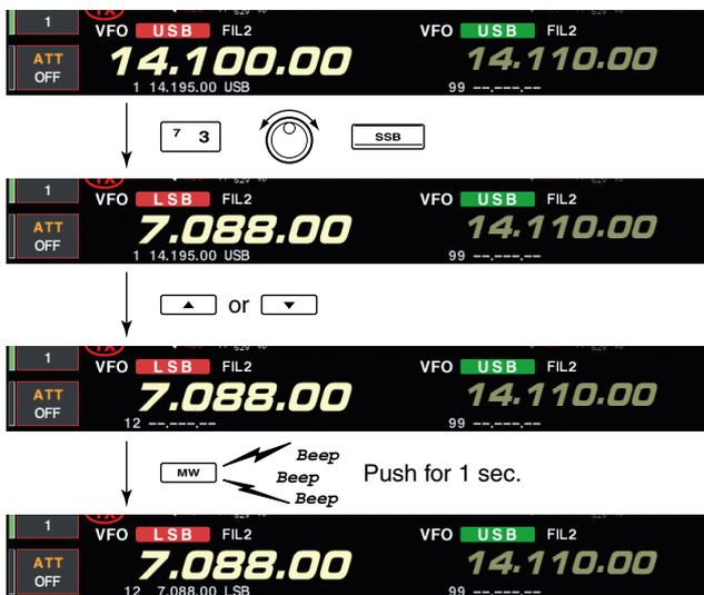
Memory channel programming can be performed either in VFO mode or in memory mode.
