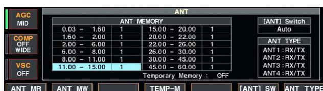
This function stores the antenna connector number for each frequency band.
