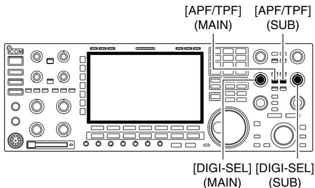
The APF changes the audio frequency response by boosting a particular frequency to enhance a desired CW signal.
