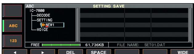
Memory channel contents, set mode settings, etc. can be saved into the CF (Compact Flash) memory card for backup.
