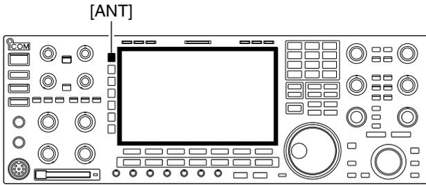
The IC-7800 has 4 antenna connectors for the HF/50 MHz bands, [ANT1], [ANT2], [ANT3], and [ANT4].
