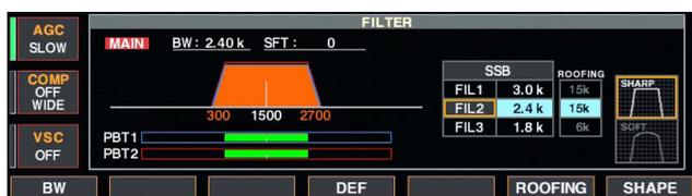
The type of DSP filter shape for each SSB, SSB data and CW can be selected independently from soft and sharp.
