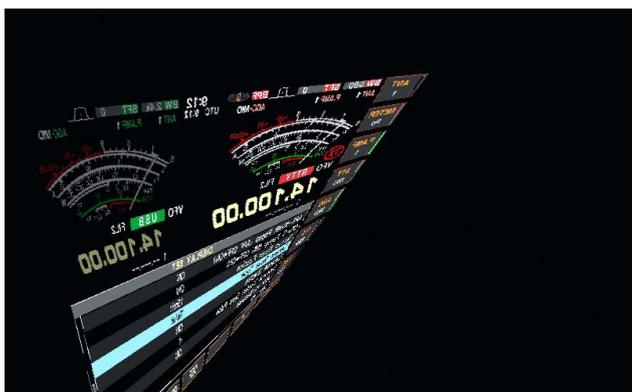
The IC-7800 has a screen saver function to protect the LCD from the “burn-in” effect.
