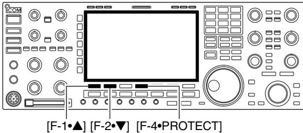
The protect function is available to protect the recorded contents from accidental erasing, such as over-record, etc.
