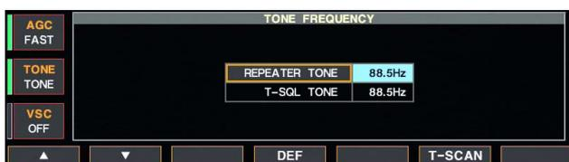
Some repeaters require subaudible tones to be accessed. Subaudible tones are superimposed over your normal signal and must be set in advance. The transceiver has 50 tones from 67.0 Hz to 254.1 Hz.
