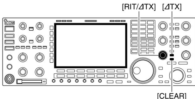
The  $\Delta$ TX function shifts the transmit frequency up to  $\pm 9.999$  kHz in 1 Hz steps (10 Hz steps when cancelling the 1 Hz step readout) without moving the receive frequency.
