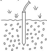
Use the heaviest gauge wire or strap available and make the connection as short as possible.
