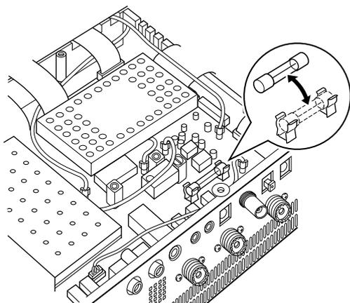
When no external DC output is available from [EXT DC] and ACC connectors, the internal fuse may be open. Replace the fuse in this case.
