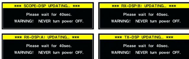
⑫ Depending on the updating, one to four dialogs as at left appears in the IC-7800 display in sequence.
