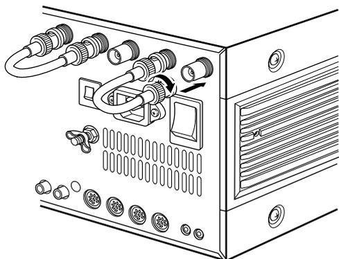
Connect the supplied coaxial cable (terminated with BNC connectors) between [RX ANT A— IN] and [RX ANT A— OUT], and, [RX ANT B— IN] and [RX ANT B— OUT], respectively.
