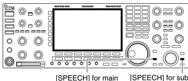
The IC-7800 has built-in voice synthesizer to announce the frequency, mode, etc. (S-meter level can also be announced—p. 12-17) in clear, electronically-generated voice, in English (or Japanese).
