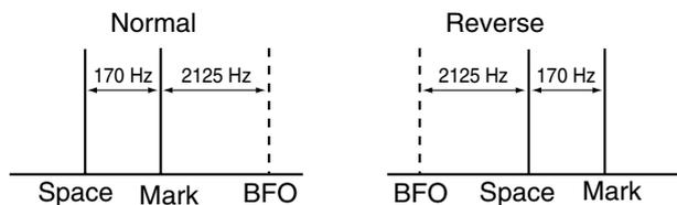
Received characters are occasionally garbled when the received signal has Mark and Space tones reversed. This reversal can be caused by incorrect TNC connections, setting, commands, etc. To receive reversed RTTY signals correctly, select RTTY-R mode.
