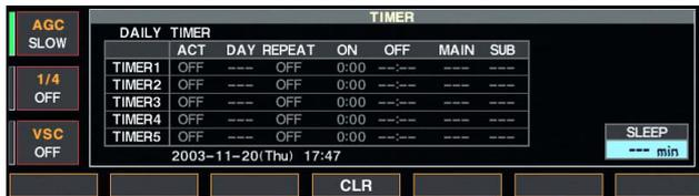
The sleep timer turns the transceiver power OFF automatically after passing the set period. The timer can be set to 5–120 min. in 5 min. steps.
