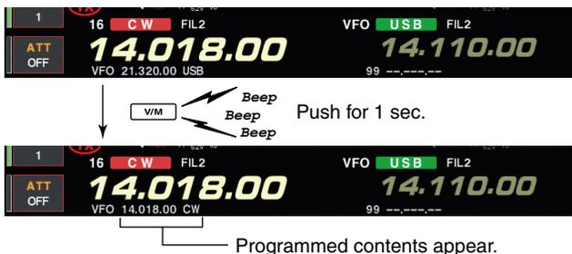
This is useful for transferring frequency and operating mode while operating in memory mode.
