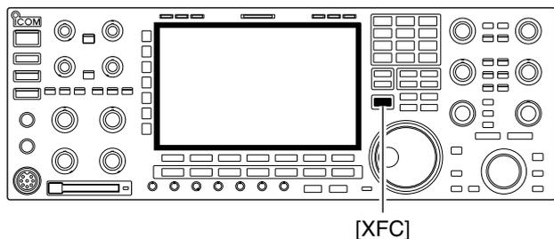
When the  $\Delta$ TX function is ON, pushing and holding [XFC] allows you to monitor the operating frequency directly.
