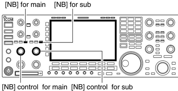
The noise blanker eliminates pulse-type noise such as the noise from car ignitions. The noise blanker is not available for FM mode.
