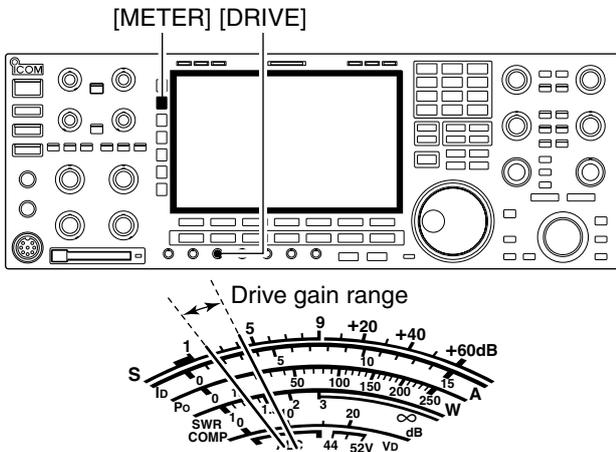
The drive gain is active for all modes except SSB without speech compressor. The [DRIVE] control adjusts the amplifying gain at the driver stage.
