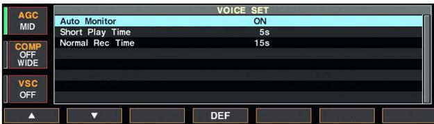
Sets the automatic monitor function, short play and normal recording times for voice recorder.
