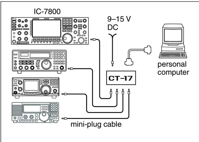
The transceiver can be connected through an optional CT-17 CI-V LEVEL CONVERTER to a PC equipped with an RS-232C port. The Icom Communications Interface-V (CI-V) controls of the transceiver.
