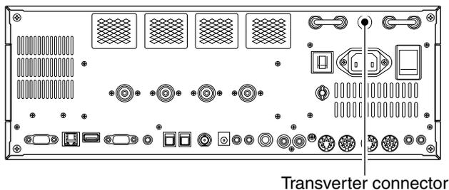
When 2 to 13.8 V is applied to pin 6 of [ACC 2], the [X-VERTER] connector is activated for transverter operation and the antenna connectors do not receive or transmit any signals. (p. 4-6)
