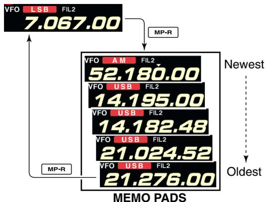
You can simply call up the desired frequency and operating mode of a memo pad by pushing [MP-R] several times.
