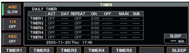
The transceiver turns power ON and/or OFF automatically on the specified day and time, with the specified frequency settings in each main and sub readout.
