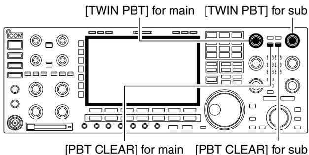
In general PBT (Passband Tuning) electronically narrows the IF passband width by shifting the IF frequency to slightly outside of the IF filter passband to reject interference. The IC-7800 uses DSP for the PBT function. Moving both [TWIN PBT] controls to the same position shifts the IF.
