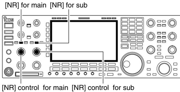
The noise reduction function reduces random noise components and enhances desired signals which are buried in noise. The DSP does the random noise reduction function.
