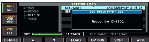
By loading the saved setting file from the CF card, you can easily set up another IC-7800— several operators settings can easily be applied to one IC-7800.
