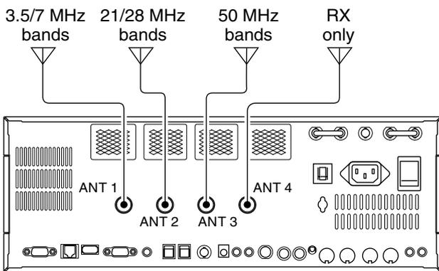
After an antenna has been selected for use (by pushing [ANT]), the antenna is automatically selected whenever that band is used.
