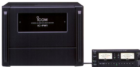
Full-duty-cycle 1 kW linear amplifier including an automatic antenna tuner. Has automatic tuning and band selection capability when used with an Icom transceiver. Full break-in (QSK) operation. The amplifier/power supply unit and the remote control unit are separate.
