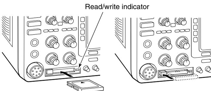
Insert the supplied CF (Compact Flash) memory card into the CF memory card slot.
