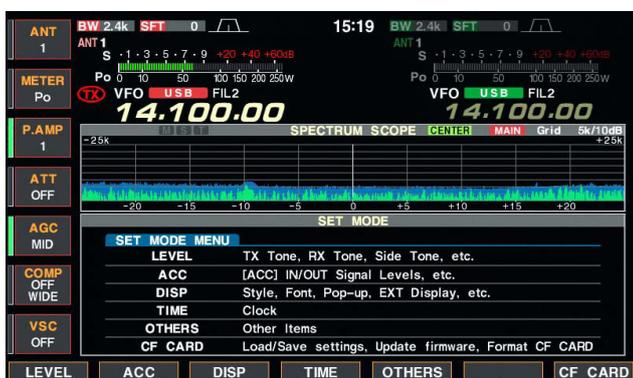
The mini scope screen can be displayed with another screen display, such as set mode menu, decoder screen, memory list screen, etc. simultaneously.
