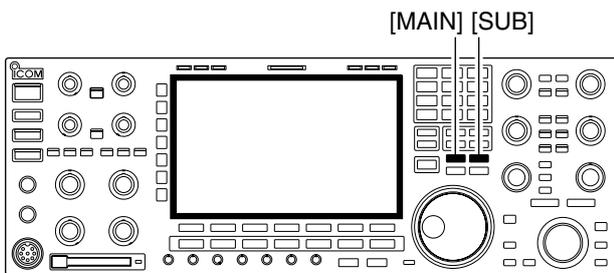
The IC-7800 has 2 identical receivers, main and sub. The main band is displayed on the left hand side, and the sub band is displayed on the right hand side of the LCD. Some functions can only be applied to the selected band and transmission occurs on the main band (except during split frequency operation).
