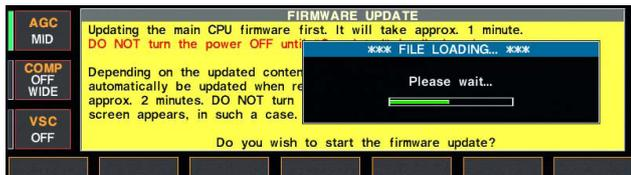
When updating the firmware using with the CF memory card, no IP address as well as subnet mask settings are necessary.
