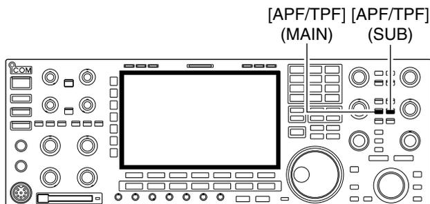
The twin peak filter changes audio frequency response by boosting the mark and space frequencies (2125 and 2295 Hz) for better reception of RTTY signals.
