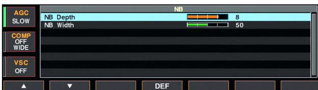
To deal with various type of noises, attenuation level and noise width can be set in NB set mode.
