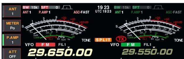
A repeater amplifies received signals and retransmits them at a different frequency. When using a repeater, the transmit frequency is shifted from the receive frequency by an offset frequency. A repeater can be accessed using split frequency operation with the shift frequency set to the repeater's offset frequency.
