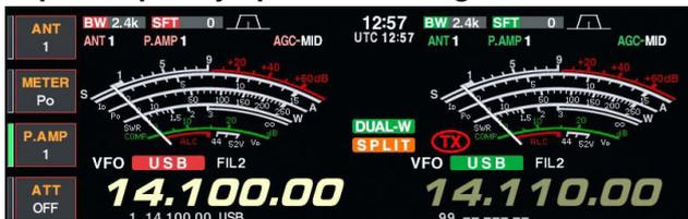
Dualwatch monitors 2 frequencies simultaneously. The IC-7800 has 2 independent receiver circuits so that you can use dualwatch with no compromises, even on different bands and modes.
