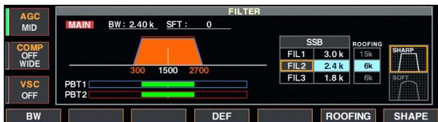
The IC-7800 has 3, 6 and 15 kHz roofing filters at the 1st IF frequency. The roofing filter provides interference reduction from nearby strong signals.
