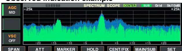
This DSP-based spectrum scope allows you to display the conditions on the selected band, as well as relative strengths of signals. The IC-7800 has two modes for the spectrum indication— one is center mode, and another one is fix mode.
